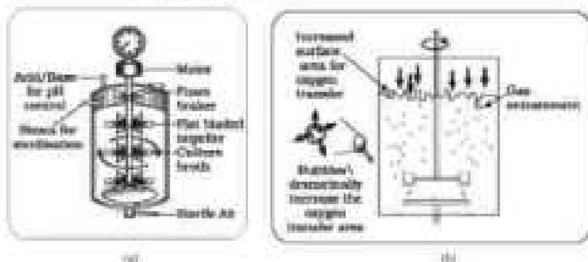
Figure 11.2 (a) Simple stirred tank bioreactor; (b) sparged stirred tank bioreactor through which sterile air bubbles are sparged.
